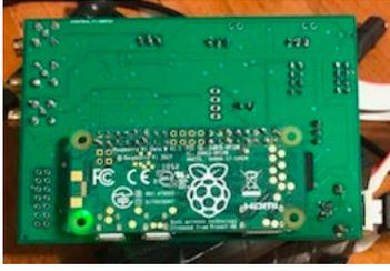
FIG. 11. Raspberry Pi Zero connected to the bottom of the finished readout board.
