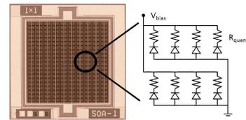
FIG. 6. Basic diagram of a SiPM.
