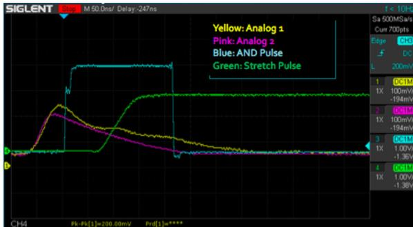
FIG. 16. Example of a basic AND pulse.
