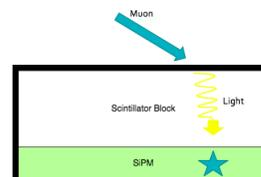
FIG. 7. Diagram of a “basic” particle detector. The muon hits the scintillator block causing a photon to be emitted. This photon is then detected by the SiPM.
