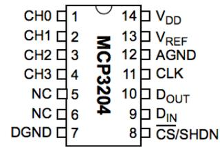
FIG. 9. The MCP3204 analog to digital converter.
