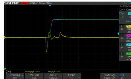
FIG. 10. Example of a oneshot pulse.
