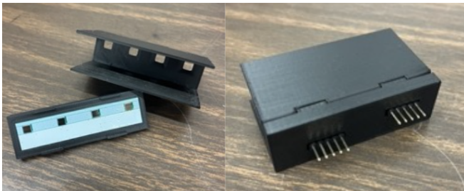
FIG. 9. A populated SiPM board placed in the mount cap and a view of the fully assembled SiPM mount.
