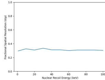
(b) Fractional spatial resolution obtained by the ratio of the standard deviation and the mean at each energy bin
