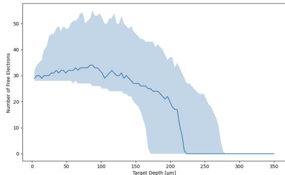
FIG. 10: Median number of free electrons produced across 500 simulations as a result of the ionization energy deposited. The number of electrons produced is found by dividing the ionization energy deposited by the energy required to ionize one argon atom (15.6 keV).
