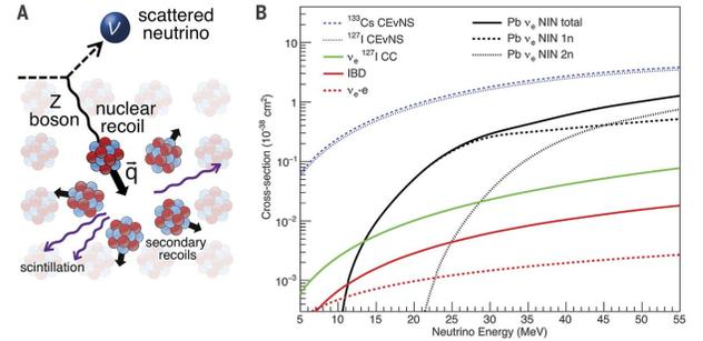
FIG. 1: A:  $\text{CE}\nu\text{NS}$  Interaction where nuclear recoil is the only detectable observable
