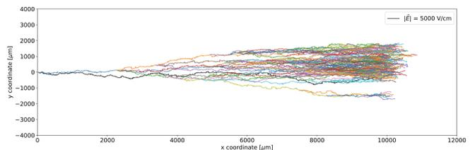
FIG. 11: TRANSLATE simulation: electrons in gaseous argon at a constant electric field of 5000 V/cm. Each branch is caused by secondary ionization where a new free electron is produced [3]
