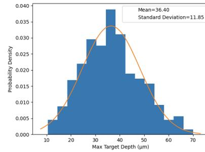
(a) Distribution of 500 simulations at an initial energy of 10 keV. Gaussian fit is used to obtain fractional spatial resolution
