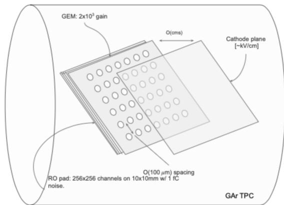
FIG. 12: Proposed GEM detector model with 100  $\mu\text{m}$  spacing between holes on GEM foil
