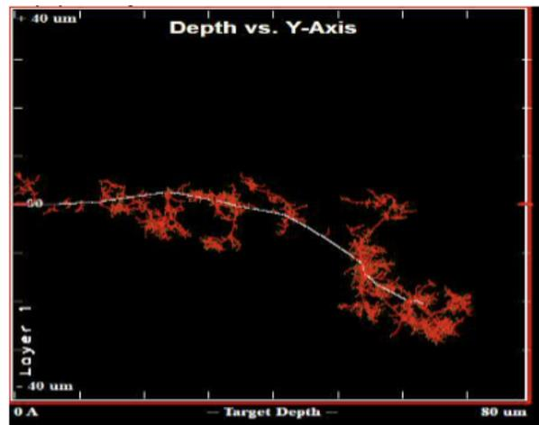
FIG. 2: Simulation of a single 30 keV nuclear recoil in gaseous argon: The white line shows the nuclear recoil trajectory, red cascades show secondary recoils
