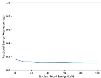
(b) Fractional energy resolution obtained by the ratio of the standard deviation to the mean at each energy distribution
