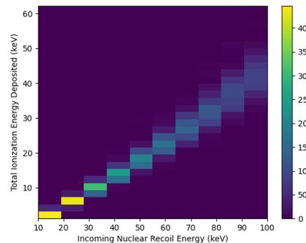
FIG. 8: Ionization energy deposited for each nuclear recoil energy. Each 10 keV bin contains 500 simulations
