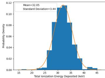
(a) Distribution of 500 simulations at an initial NR energy at 70 keV. Gaussian fit is used to obtain fractional energy resolution
