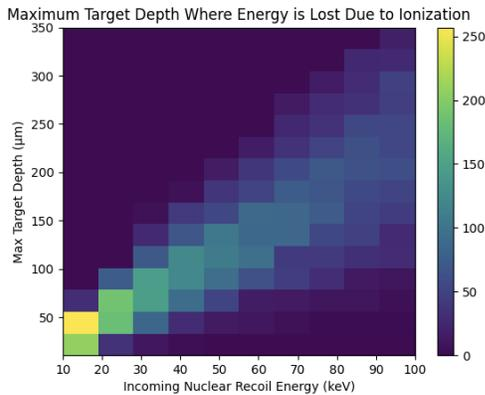
FIG. 6: Size of ionization signatures for each initial nuclear recoil energy. Each 10 keV bin contains 500 simulations
