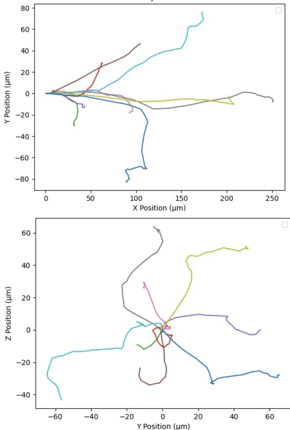
FIG. 3: *Upper:* 1-100 keV nuclear recoil trajectories projected on XY plane. Each trajectory color corresponds with a different recoil energy. This plot follows the nuclear recoil trajectory along the target depth
