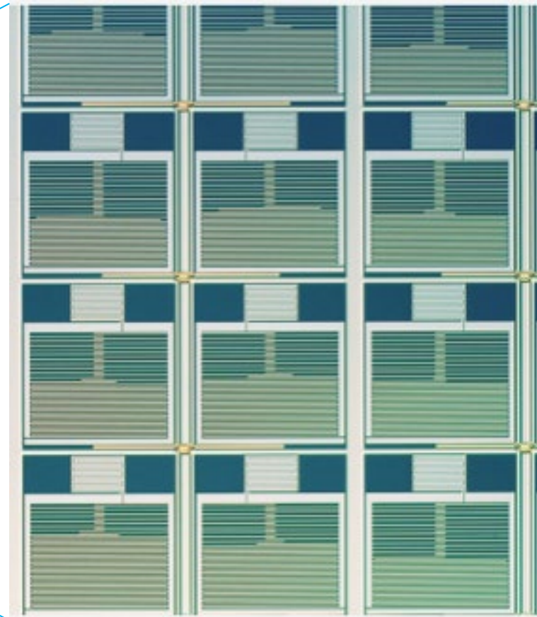
Microscopic view of individual MKIDs (pixels)
